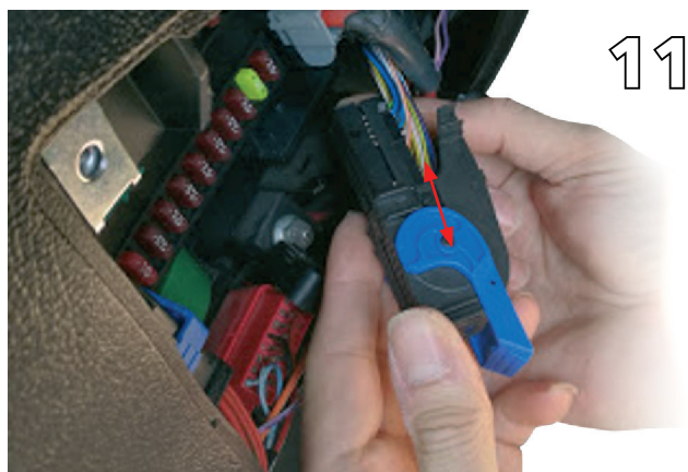
Remove the black connector and slide open
